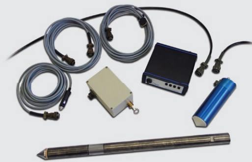
Basic components of the RW NOVA CPT system (clockwise from the left): Instrumentation Cords, Depth Encoder, Computer Interface, RW NOVA Receiver, and RW NOVA Transmitter assembled to the NOVA CPT Probe.
