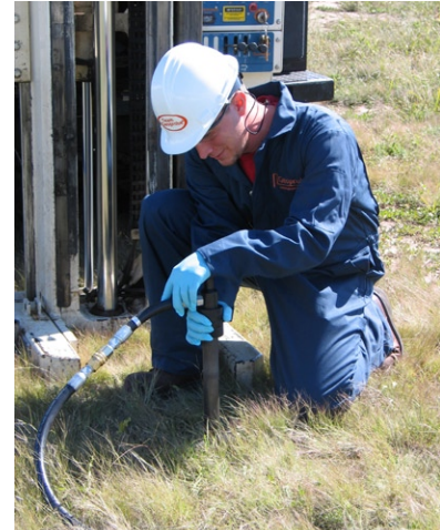
The GS2200 is also capable of delivering standard ASTM grout mixes or for injecting harsh remediation materials.
