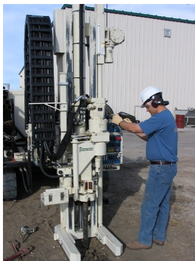
(above) A 1.25 in. light-weight center rod is added to the tool string. (right) A MC 5 tool string is driven to depth using a Geoprobe ® 7730DT machine.
