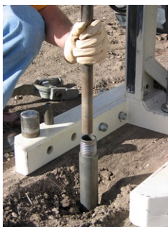
(above) A 1.25 in. light-weight center rod is added to the tool string. (right) A MC 5 tool string is driven to depth using a Geoprobe ® 7730DT machine.
