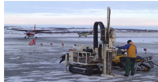
Some of the testing done for Macro-Core ® Center Rod System was completed through ice lenses and permafrost. The durability of the system allowed field operators to probe in much tougher soils. Fewer parts speed up decontamination and re-assembly of the sampler which increases the footage/production rate.
