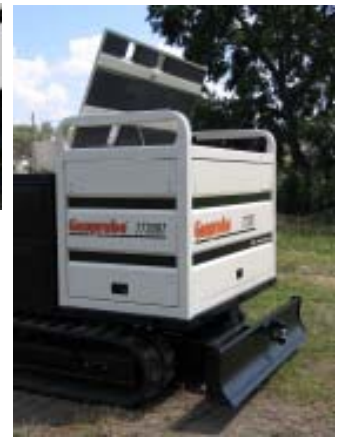
(right) Four swing-open doors allow easy access for daily maintenance to the engine and hydraulic components.
