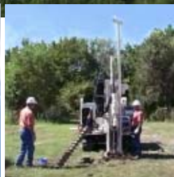
(far left) Two-speed augerhead, overhead mast, hydraulic winch, and GH60 hamer.
