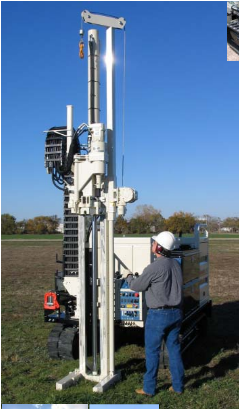
(far left) Two-speed augerhead, overhead mast, hydraulic winch, and GH60 hamer.
