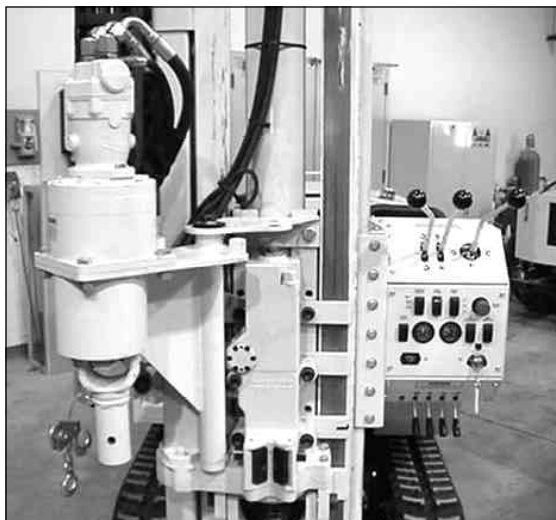
Figure 1. Augerhead rotated to access hammer.
