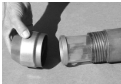
(left) RS60 Cutting Shoe (15390), RS60 Spacer Ring (16410), RS60 PVC Liner, and 3.26 in. Probe Rod.
